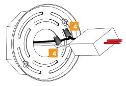
Install glass via three thumb screws in an accessory bag.
